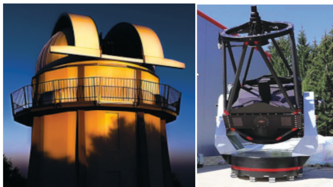
Figure 1: Left, the pavilion for the 140cm telescope. Right, the telescope while it was still in the ASA company.
